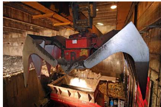
(1) AUTOMATIC BRIDGE CRANE SPIDER ™ FOR MATERIAL HANDLING
