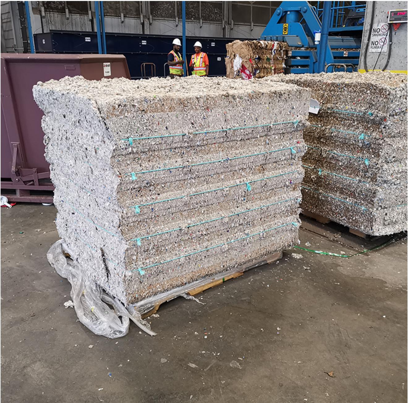
So, along came a more processed product called engineered fuel with less moisture, higher heat value and more consistent quality. Also known as solid recovered fuel (SRF), depending on quality and process, it can replace up to 100 percent of fossil fuels to generate electricity or heat. Though it is more often in the range of 30 to 60 percent. End users are typically operators of cement kilns and boilers.
